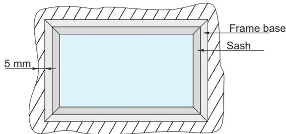
Subtract a minimum of 5mm from the dimensions of the height and width of the cavity in the wall.
