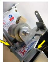
Remove the cap and put the cable gland in place.
