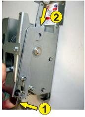
Put the spool in place in the upper part of the winch. Check the plate is securely fitted inside the encasement. Use the screw supplied.
